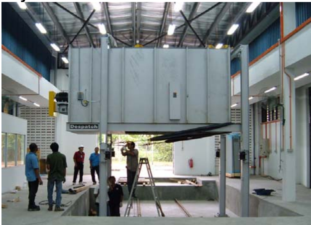
Figure 2: The furnace body is raised and secured between the four furnace columns.
